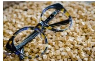
TCN offers a complete range of polishing pastes for a dry-barreling process, especially efficient on cellulose acetate material.
