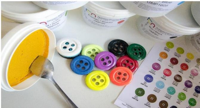
**GMP dyeing pastes** are used at a concentration of **0.5 to 5 g/l** at **95°C**.
